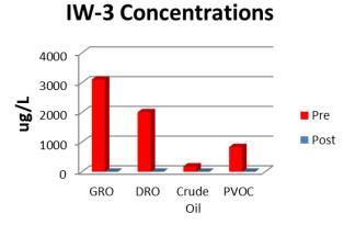
**Project Results:** Three rounds of sampling have occurred during the post treatment period with non-detect results for all COC's sampled at IW-2 and IW-3. The results yield a 100% reduction for contaminant levels at IW-2 and IW-3. The use of vacuum extraction helped to distribute the treatment chemistry to ensure complete coverage in the target area of concern. ORIN is currently conducing full-scale injection at this site.
